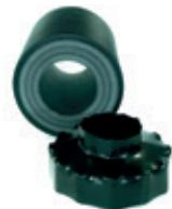
Reducing adapters are used to accommodate smaller pipe diameters in larger insulation kit inlets. The reducing adapter is pressed into the insulation kit and the transition between the adapter and the pre-insulated pipe is sealed with the heat shrink end cap, included in the set.
