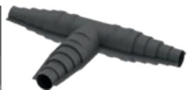
Watertight HDPE buried insulation kit for T-junctions between single, double or quadruple pre-insulated pipes. Comes complete with mineral wool insulation, sealing compound, stainless steel bolts and plates and mounting instructions.
